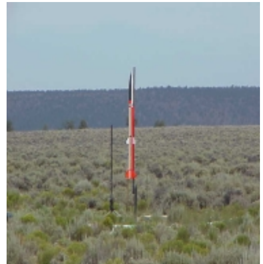
My 5.5" Doorknob is ready to launch outside of Brothers, OR, on a K700/J415/H128 combo.
