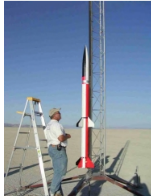
Kent Newman with the "Doorknob" on a KBA K600 to a K185 to (2) H128s. The flight was successful to 7145' and had a nominal recovery.
